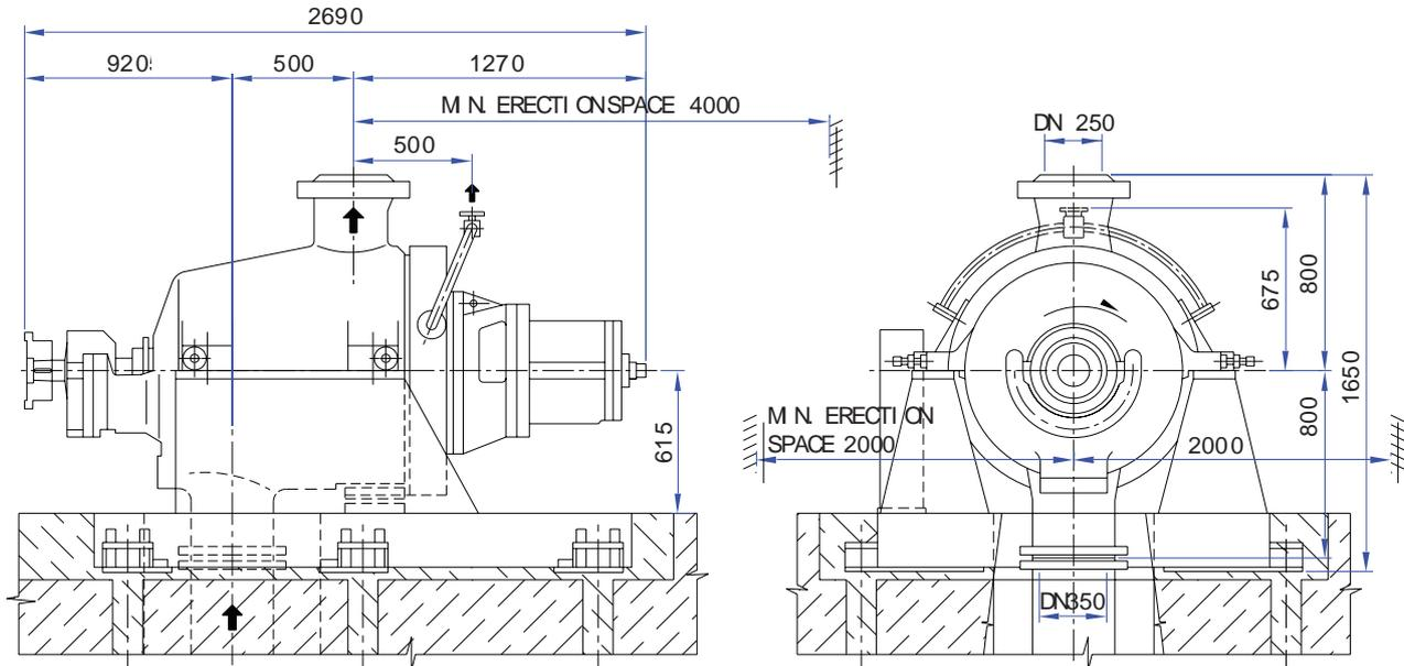
Suction branch flange is machine, with raised face, PN on request.
